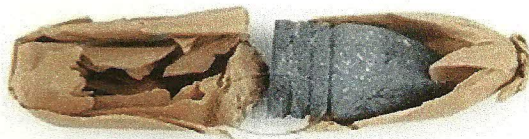
Fig. 12. Confederate .58-cal cartridge, date unknown. Note the internal powder cylinder and the pasted end of the powder case.
