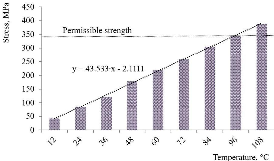
**Fig.11** Dependence of the maximum equivalent stresses in the container from the temperature of the cargo transported in it
