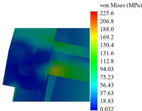
**Fig.8** The stresses distribution in the container structure when it is loaded with inertial forces in the longitudinal direction following the movement of a semi-trailer
