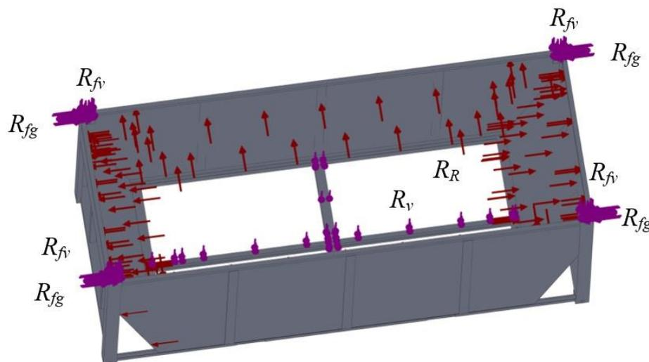
**Fig.5** A calculation diagram of the container during lifting for upper corner fittings
