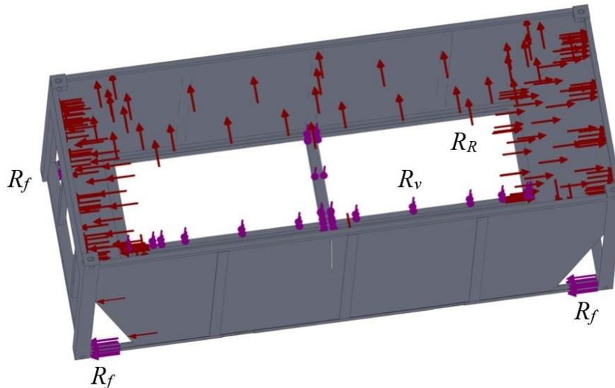
**Fig.7** A calculation diagram of the container when it is loaded with inertial forces in the longitudinal direction following the movement of a semi-trailer
