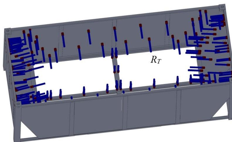
**Fig.10** A scheme of application of the temperature load to the inner surfaces of the container
