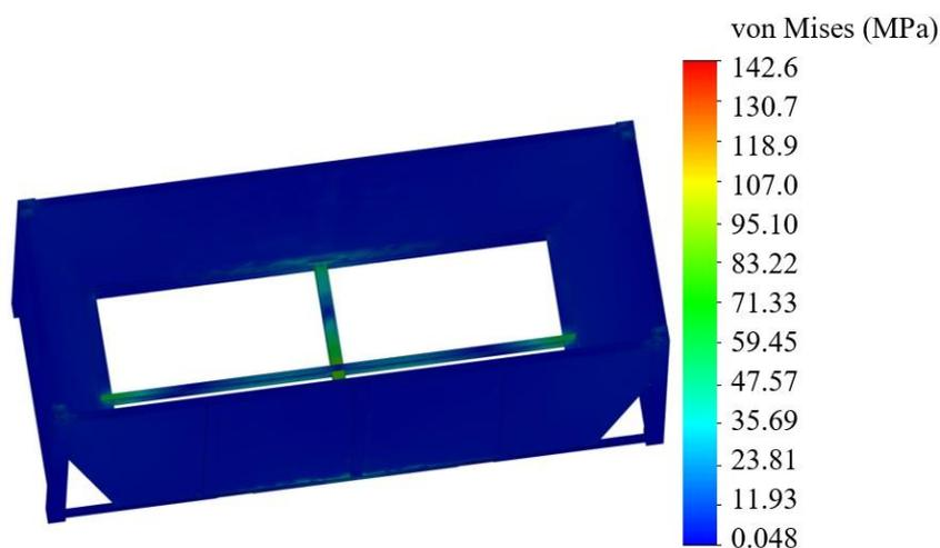
**Fig.6** The stresses distribution in the container structure during lifting
