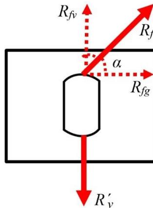
**Fig.4** A scheme of force action on the upper fitting of the container
