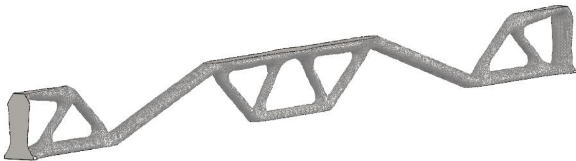
Fig. 6 Topology optimization from Siemens NX software Source: (authors)
