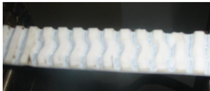
Fig. 6 Borderline deformation of a toothed belt connection 1(finger welding).
