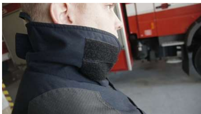
Fig. 6 Neck area - critical place for heat penetration
